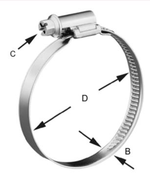
C (screw type) = C7 - 7mmDiameter D = 190-210Width B = 12.0
